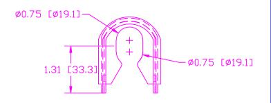
MATERIAL: CLEAR PVC 95 DUROMETER (SHORE A) TOLERANCE UNLESS OTHERWISE SPECIFIED: ±.030"/±0.8mm RADIAL DIAMETERS TO BE MEASURED OVER MANDRELS, RING GAGES OR PIN GAGES OF SUITABLE SIZE
