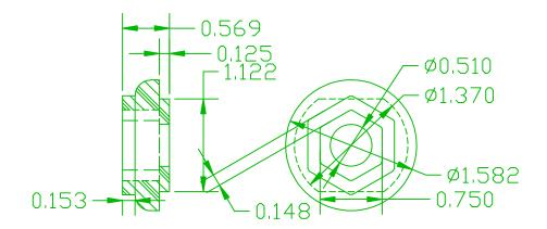
BASE MATERIAL: BASE MATERIAL U.L. RATING: 25% GLASS-REINFORCED NYLON 94 V-0
