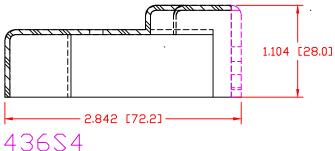
DESIGNED TO FIT 16 OR 25 mm<sup>2</sup> METRIC CABLE FITS THE FOLLOWING BATTERIES:
