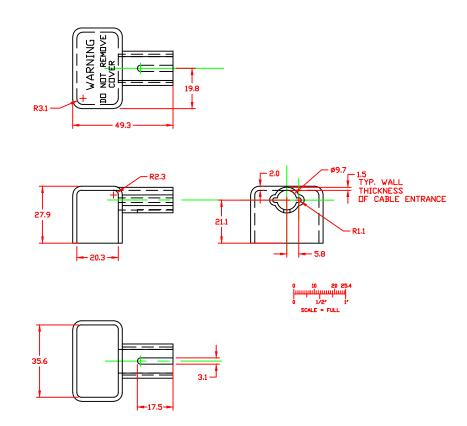
TOLERANCE UNLESS OTHERWISE SPECIFIED: ±.030"/±0.8mm RADIAL DIAMETERS TO BE MEASURED OVER MANDRELS, RING GAGES OR PIN GAGES OF SUITABLE SIZE
