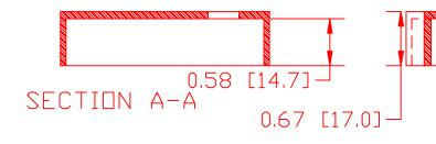
TOLERANCE UNLESS OTHERWISE SPECIFIED: ±.030"/±0.8mm RADIAL DIAMETERS TO BE MEASURED OVER MANDRELS, RING GAGES OR PIN GAGES OF SUITABLE SIZE
