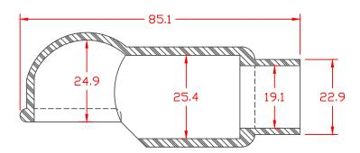
TOLERANCE UNLESS OTHERWISE SPECIFIED: ±.030'/±0.8mm RADIAL DIAMETERS TO BE MEASURED OVER MANDRELS, RING GAGES OR PIN GAGES OF SUITABLE SIZE
