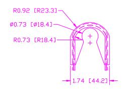
TOLERANCE UNLESS OTHERWISE SPECIFIED: ±.030"/±0.8mm RADIAL DIAMETERS TO BE MEASURED OVER MANDRELS, RING GAGES OR PIN GAGES OF SUITABLE SIZE
