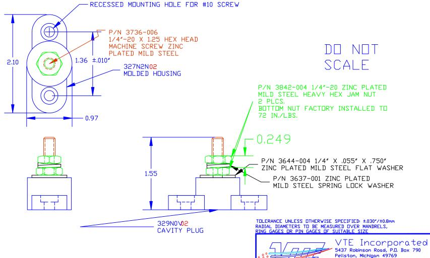
BASE MATERIAL: BASE MATERIAL U.L. RATING: DIELECTRIC STRENGTH: VOLTAGE RATING: CURRENT RATING: TEMP. RISE AT LOAD: 52 DEG. F. MAXIMUM RECOMMENDED TORQUE: 60 IN./LBS.
