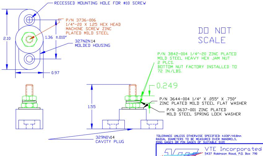
BASE MATERIAL: BASE MATERIAL U.L. RATING: DIELECTRIC STRENGTH: CURRENT RATING: TEMP, RISE AT LOAD: MAXIMUM RECOMMENDED TORQUE: 60 IN./LBS.
