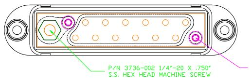
P/N 3872 #8-16 TORX PLUS THREAD FORMING SCREW (2 REQ'D)
