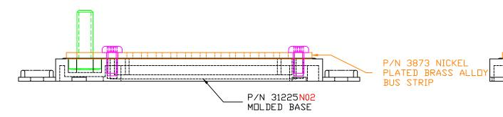
TOLERANCE UNLESS OTHERWISE SPECIFIED: ±.030"/±0.8mm RADIAL DIAMETERS TO BE MEASURED OVER MANDRELS, RING GAGES OR PIN GAGES OF SUITABLE SIZE
