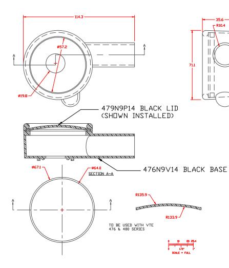
BASE HOUSING MATERIAL: LID MATERIAL: BLACK PVC BLACK POLYPROPYLENE TOLERANCE UNLESS OTHERWISE SPECIFIED: ±.030"/±0.8mm RADIAL DIAMETERS TO BE MEASURED OVER MANDRELS, RING GAGES OR PIN GAGES OF SUITABLE SIZE
