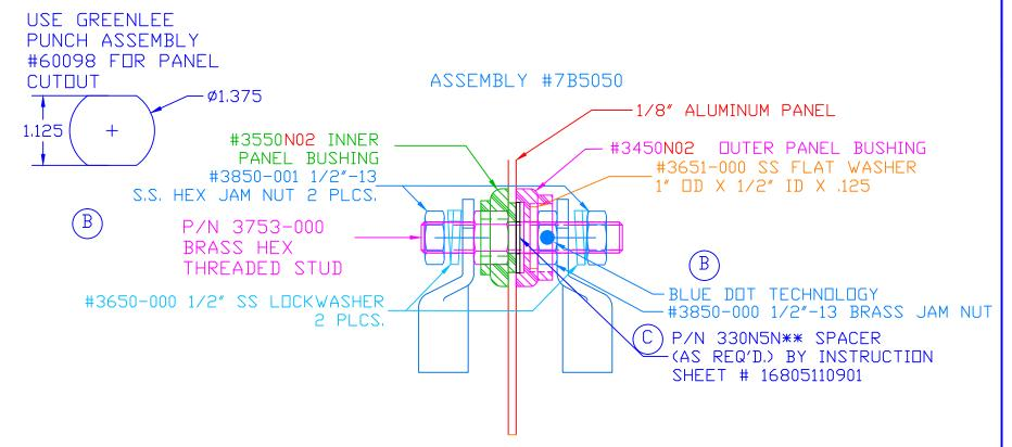
INCLUDES P-16808110001 BLUE DOT MULTI LABEL, 1 PER CONTAINER MAXIMUM AMPERAGE: 500 AMPS @ 12VDC MAXIMUM RECOMMENDED FASTENER TORQUE:
