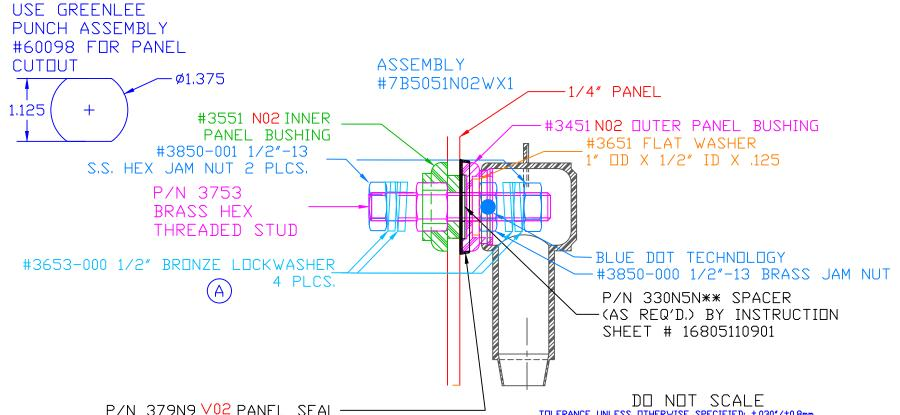
INCLUDES P-16808110001 BLUE DOT MULTI LABEL, 1 PER CONTAINER MAXIMUM AMPERAGE: 500 AMPS @ 12VDC
