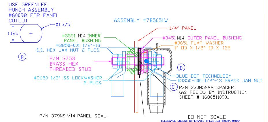
INCLUDES P-16808110001 BLUE DOT MULTI LABEL, 1 PER CONTAINER MAXIMUM AMPERAGE: 500 AMPS @ 12VDC
