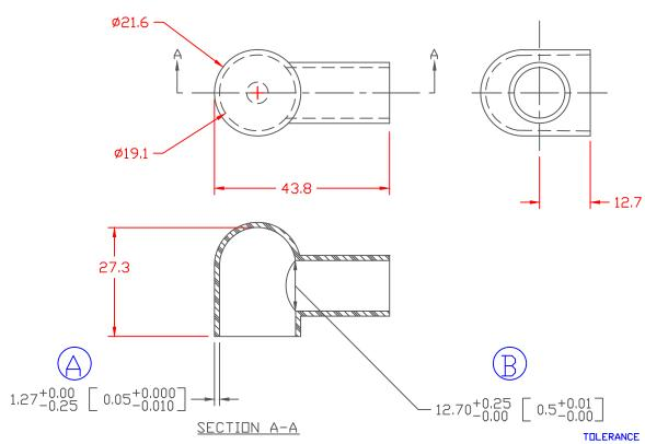
TOLERANCE UNLESS OTHERWISE SPECIFIED: ±.030"/±0.8mm RADIAL DIAMETERS TO BE MEASURED OVER MANDRELS, RING GAGES OR PIN GAGES OF SUITABLE SIZE
