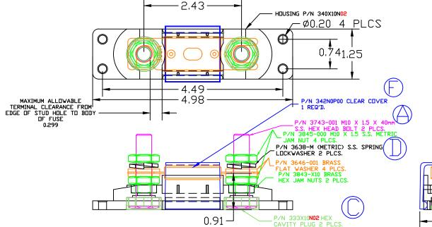
MAXIMUM RECOMMENDED AMPERAGE: 300 AMPS @ 12 VDC
