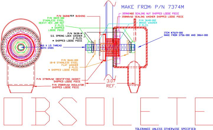
MAXIMUM FASTENER TORQUES: JAM NUTS: 15 FT./LBS. (180 IN./LBS.) SEALING NUT: 10 FT./LBS. (120 IN./LBS.)
