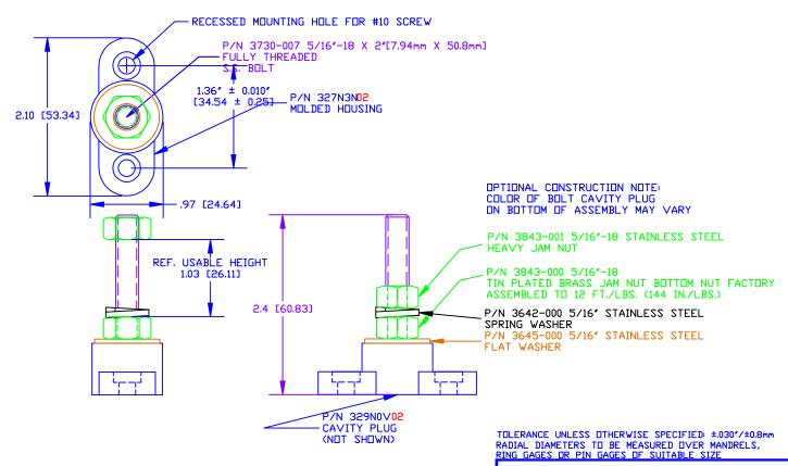
BASE MATERIAL: BASE MATERIAL U.L. RATING: DIELECTRIC STRENGTH: CURRENT RATING: TEMP, RISE AT LOAD:
