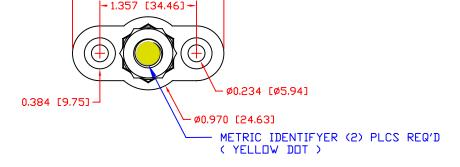
MATERIAL PART NO: MATERIAL: VENDOR PART NO: SPECIFIC GRAVITY: MELTING TEMP: U.L. RATING: 7111210502 GLASS FILLED NYLON HYLON N2015 HL NAT 1.23 515 F [268 C] UL 94 HB
