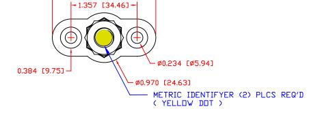
MATERIAL PART NO: MATERIAL: VENDOR PART NO: SPECIFIC GRAVITY: MELTING TEMP: U.L. RATING: 1111210514UL GLASS FILLED NYLON HYLON N2015 HL BK 1.23 1.25 F [268 C] UL 94 HB
